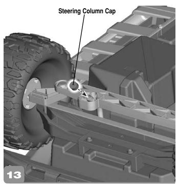
• Fit the steering column cap onto the end of the steering column.
